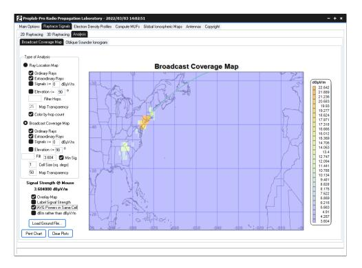
The results above indicate that there is a fairly large area along the east coast of the United States where it might be possible to pick up the backscattered signal. Note in the legend on the right that the minimum signal level plotted is about 3 dB microvolts per meter, which is near the noise floor.
