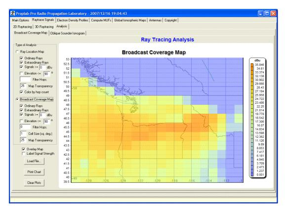
Notice that the line of focusing has indeed boosted field strength from southwestern Montana through northern Oregon. To determine what aspect of the ionospheric (or perhaps tilted ground?) reflections is responsible for that enhancement would require additional study of the signal rays themselves, which we will leave as an exercise for the reader.
