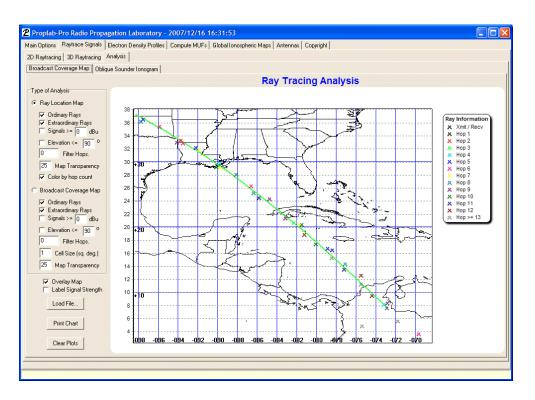
No additional significant deviations occur over the relatively flat land of the southern U.S., but the small deviations that occurred over the northern Rocky Mountains are causing additional signal spreading the further the signal travels.
