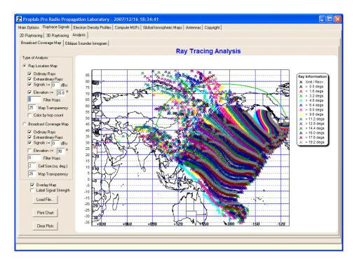
Including only elevation angles of less than or equal to 20.8 degrees, the map changes as shown. We can see that the southern-most band of enhanced signals from just north of New Zealand and through the northern reaches of Indonesia involve signals with very low elevation angles of a little more than 4.8 degrees.
