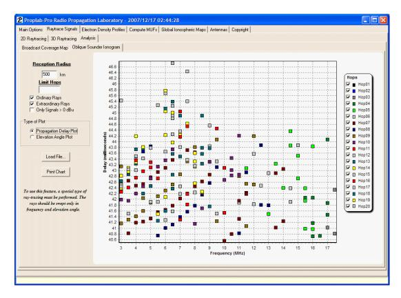
This is a propagation delay plot of the same data. It shows how long it takes signals of varying frequencies and elevation angles to reach the receiver and is important because it helps identify multipathing effects and resultant signal distortion. For modem-based radio communications, this information can be used to help define the limits of communications speed on various paths.
