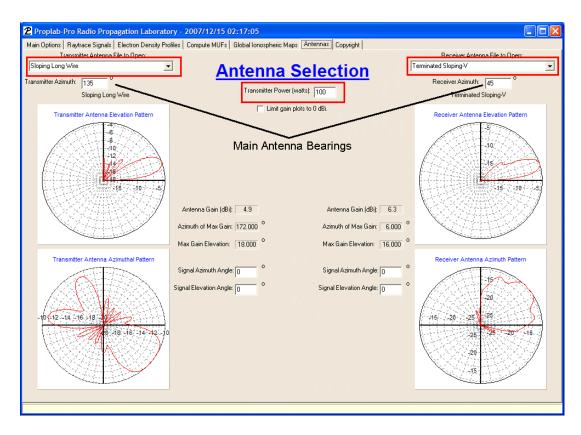
The three most important boxes are highlighted. The left-hand drop-down box lets you select a transmitter antenna radiation pattern from the antenna files located in the ANTENNAS folder. The right-side box lets you choose the radiation pattern for the receiver. The center box is where you specify the radiated power of the transmitter, in watts.
