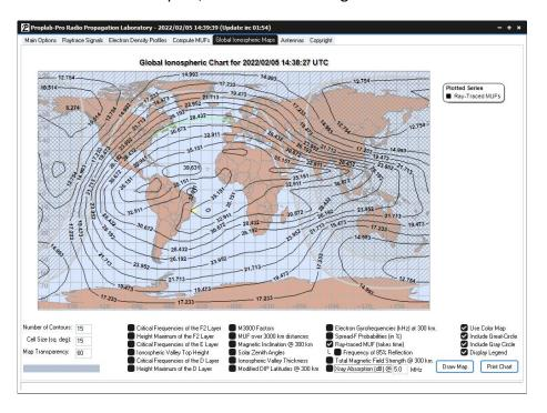
This indicates our MUF should be near 28 MHz. Let's choose a frequency a little lower to ensure that our signal gets there without significant attenuation, since this is a daylight path. Let's use 15 MHz as our transmitter frequency.
