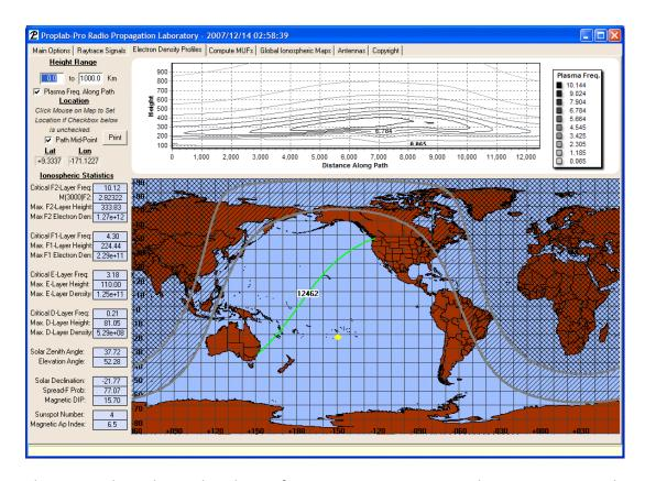
The upper chart shows the plasma frequency contours across the entire great-circle path from Seattle to Sydney. This is particularly useful information to the radio communications specialist because it shows how the ionospheric layers are tilted. Tilts in the ionospheric layers can cause non-great-circle propagation and other odd behavior such as chordal hops, etc. This chart can therefore help you diagnose potential propagation anomalies without requiring any ray-tracing at all.
