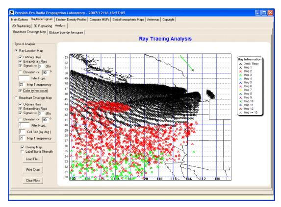
This is a zoomed in view showing signals of varying hop counts and filtered to field strengths of greater than or equal to zero  $dB\mu V/m$  (with a 50 ohm system) from the example above.
