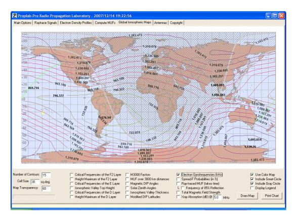
Electrons gyrate around the Earth's magnetic field at a frequency that depends on the strength of the Earth's magnetic field. This is important, particularly on low radio frequencies, because the gyration can produce stronger than usual absorption and other effects. The contours represent areas of equal gyrofrequency in Hertz (Hz).
