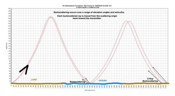
That backward reflection consumes a fraction of the energy that is reflected forward toward the receiver. As a result, backscattered signals are usually much weaker, washed out, and/or variable in nature. In many cases, the backscattered signal may be lower than the background noise and will not be detectable. However, using Proplab-Pro, an evaluation of the backscattered signals can be estimated over a range of user-selectable scenarios.
