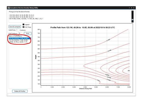
In this example, we clicked on the first profile. This great-circle path is a little over 8,000 km in length from Vancouver to Europe. Notice that the UTC date and time is set to real-time in the Main Options window of our example, so the current date and time is used for this slice.
