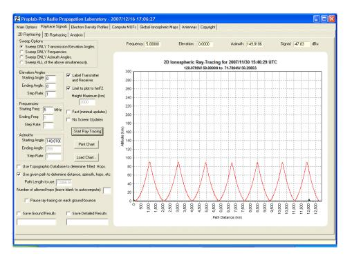
This is an example of a signal that was ray-traced **without** the topographic tilted hop feature. Notice that the signal is reflected nice and evenly from the ground to the lower E-region where it was reflected. Compare this to the results below where tilts are turned **on**.
