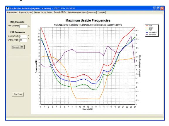
The left-side axis refers to the MUF, EMUF, FOT and normal FOT. The right-side axis refers only to the elevation angle. The UTC hour is at the base of the chart.
