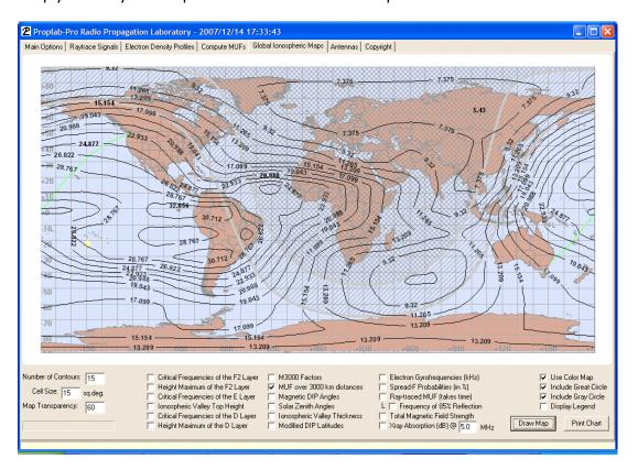
This map shows the maximum useable frequency for 3,000 km path midpoints. In other words, the contour at any specific point is the MUF for any path whose midpoint resides at that contour location.
