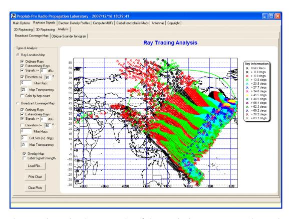
This map shows the elevation angles of the signals that are transmitted to each reception location. It is interesting to see how signals with transmitted elevation angles of greater than 6.9 degrees and less than 20.8 degrees dominate the picture. This suggests that most of the signal energy observed at ground locations is of a relatively narrow elevation angle range. Fortunately, this is within the limits of our transmitters' main elevation gain lobe.
