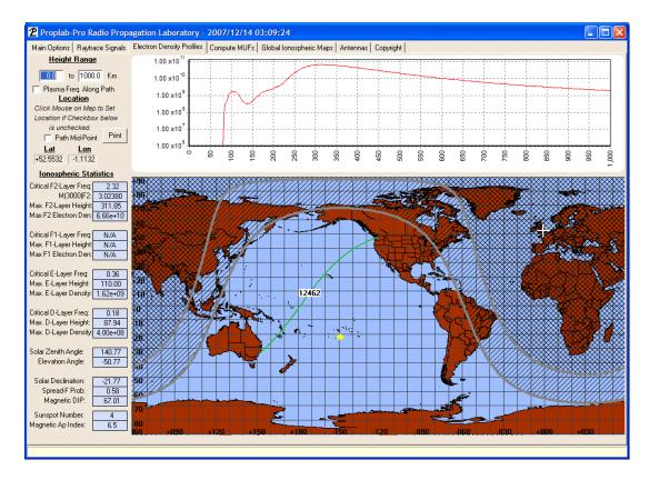
This chart was produced at the point where the white "plus" sign is located on the map over the United Kingdom. To produce this map, we UN-checked the "Path Midpoint" box and then used our mouse to click on the UK region. Once we clicked our mouse, the electron density profile for that location was computed and displayed on the chart at the top.
