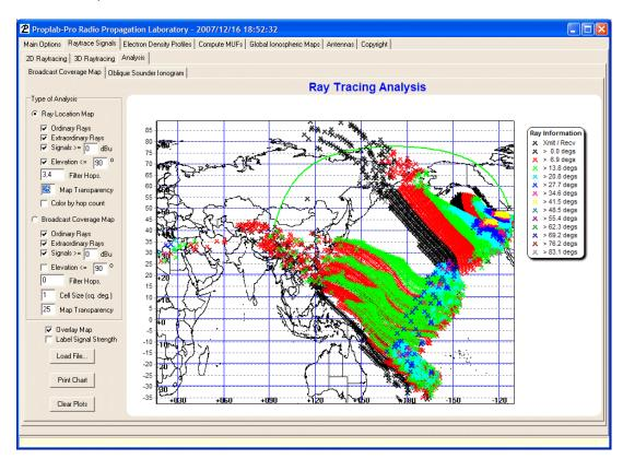
In the box labeled "Filter Hops", notice that a string of "3,4" was typed. This has told Proplab to filter out signals having hop counts of either 3 or 4.
