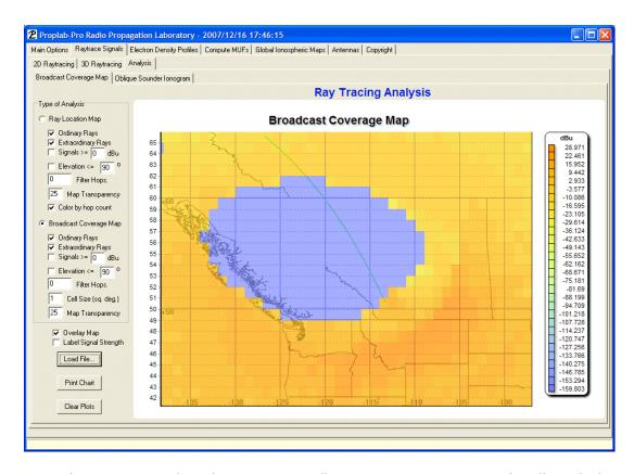
From this image, it is clear that even vertically propagation 5 MHz signals will reach the ground immediately around the transmitter with respectable strength. Thus, 5 MHz propagation is possible everywhere toward the southeast for some distance.
