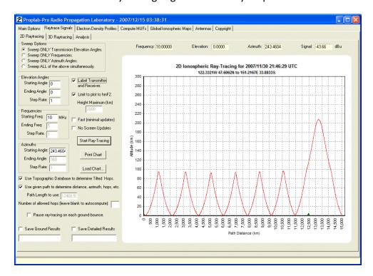
Here is a sample ray-tracing on 10 MHz between Seattle and Sydney on the date specified on the chart and using a take-off (elevation) angle of zero degrees along an azimuth of 243.46 degrees. The receiver is identified by the small triangle 12,500 km down-range. The transmitter and receiver are depicted as triangles when the "Label Transmitter and Receiver" checkbox is checked.
