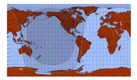
The complexity of the profile is due to the slice being made through the equatorial night zone, as well as through the equatorial day-zone where electron densities and critical frequencies peak.
