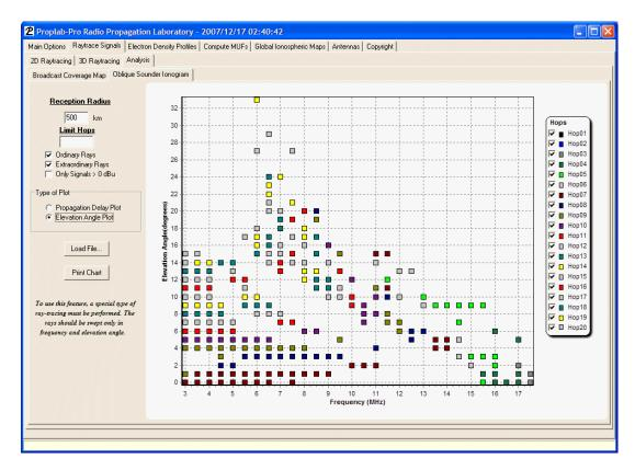
These results were obtained over the Seattle to Sydney path discussed earlier in this manual, using a frequency that was varied from 3 MHz to 30 MHz at step intervals of 0.5 MHz and elevation angles that were swept from 0 to 40 degrees in 1 degree steps.
