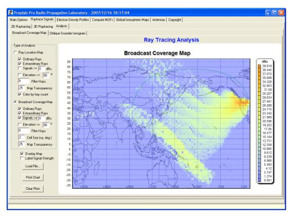
In this example, we have filtered out all signals that have field strengths of **less than** 0 dB $\mu$ V/m (with a 50 ohm system). This removes a considerable number of the rays from the results. In fact, it reveals that almost all but the northwest continental United States and the southwest corner of Canada are able to receive anything with strengths above zero dB $\mu$ V/m. Again, notice the impact of the skip zone as a focusing agent.
