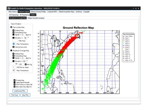
The color above represents which rays hopped once or twice from the backscattered region. NOTE: The legend says "Hop 3" is in green, but this is the second hop AFTER the signal was backscattered. The backscattering counts as one hop, so in reality, the signal has actually bounced from the ocean/ground three times since leaving the transmitter. So the chart above is correct for two backscattered bounces.
