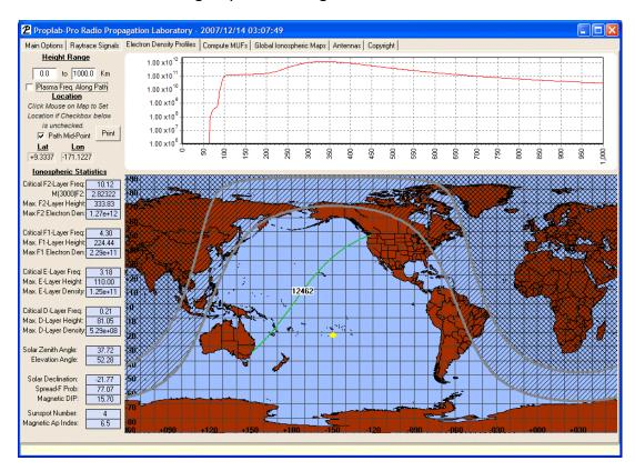
This chart shows what happens if you UN-check the "Plasma Freq. Along Path" checkbox. Notice how the top graph has changed. It now represents the vertical electron density profile over the path mid-point (because the "Path Midpoint" checkbox is checked).
