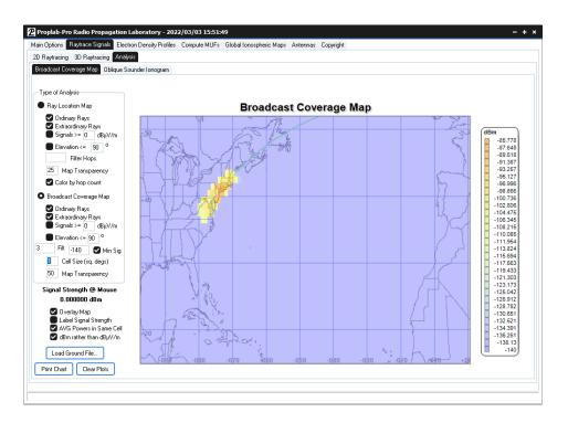
As expected, the region of highest backscattered signal field strength maps back to the area around our transmitter, since the radio path is fairly stable and supports two-way paths.
