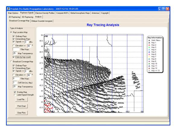
At this even deeper level of detail, you can see not only the area of signal focusing associated with the skip zone, but another interesting line of focusing that occurs from southwestern Montana through northern to north-central Oregon. Enhanced field strength and/or improved signal stability could be expected in those areas, at least for the snapshot in time that this ray-tracing session is valid for.
