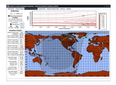
Imagine taking a knife and cutting a single line through the ionosphere along the great-circle path in green from Vancouver to Europe. At this particular date and time, and using the existing sunspot number and solar flux information that is defined in the Main Options / IRI Model Options tab, the electron density profile is plotted as plasma frequencies in the top contour map.
