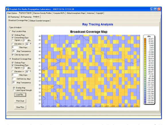
The great-circle path ends at the receiver location, which shows a box where no field strength is detected. However, remember that we're using ray-tracing, so each and every colored box represents a signal that passes close to the receiver. If we had used a smaller stepping increment in our ray-tracing phase (we used 1 degree in elevation and 1 degree in azimuth), many of these "holes" would have been filled in with signals of similar strength.
