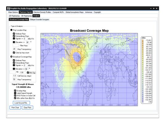
This example was obtained by saving the ground results of a ray-tracing session that varied the ray azimuth by 0.5 degrees per step in a 360 degree circle, with the elevation angle varying from 0 to 89 degrees.
