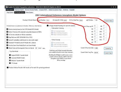
The top three numbers (running 12-month mean SSN, IG Index and solar flux) are the most important parameters, depending on the IRI model options you have chosen.
