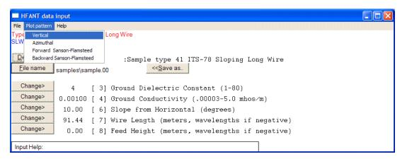
After you have selected an antenna, click on the "Plot pattern" menu option and select the "Azimuthal" choice. An azimuthal radiation pattern for that antenna will be displayed on your screen.
