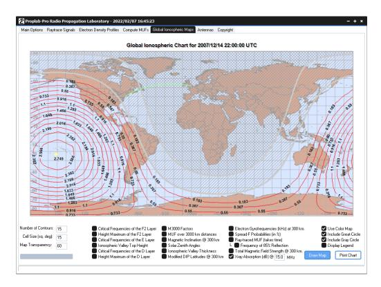
For this chart, we assumed that a powerful class X1.0 solar x-ray flare was in-progress at the time the chart was plotted. The map shows the contours of radio signal absorption (in dB) at a frequency of 15 MHz (see the box to the right of the X-ray Absorption checkbox). You can see that this event would have had a fairly substantial impact on our radio path if our signal would have been transpacific instead of transatlantic.
