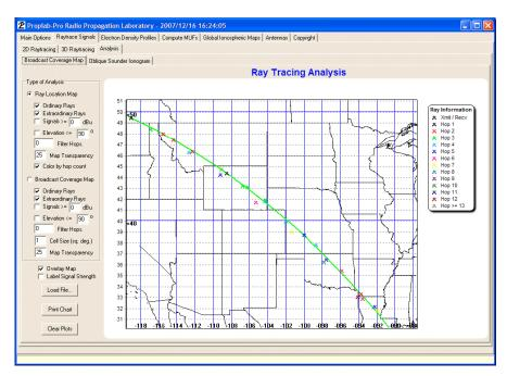
Now we zoom in over the United States where the signal starts to bounce off of tilted ground surfaces and deviate from the great-circle path. But notice that no significant tilts were hit because the deviations are still relatively small.
